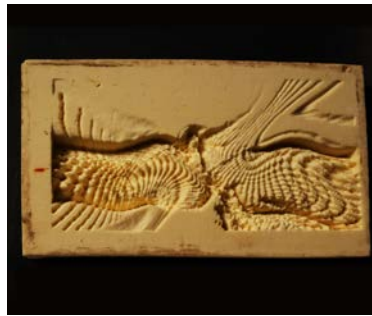
fig 6. The negative plaster of Paris mold just released from the positive modelling foam mold (right)
